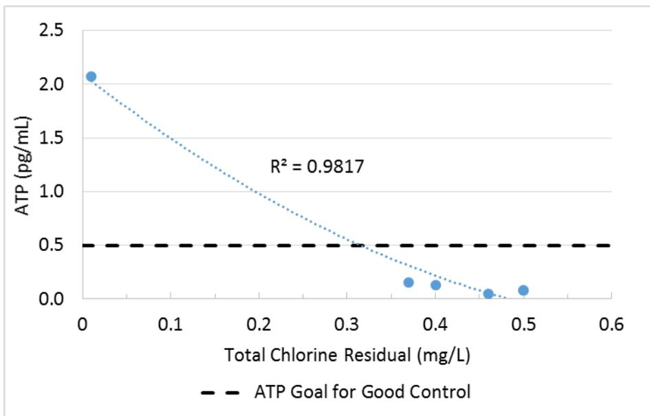
Figure 10. Total chlorine vs. ATP for Home A.
